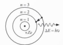
Bohr correctly proposed that the energy and radii of the orbits of electrons in atoms are quantized, with energy for transitions between orbits given by
