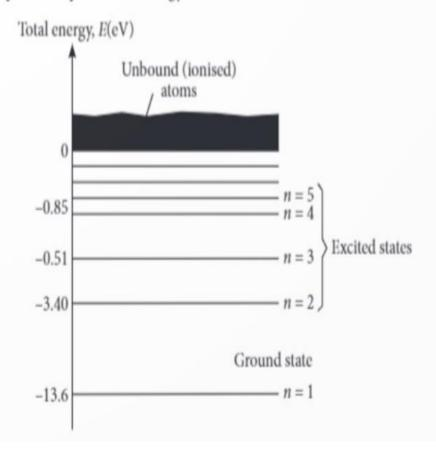
In a mixture of H—He<sup>+</sup> gas (He<sup>+</sup> is single ionized He atom), H-atoms and He<sup>+</sup> ions are excited to their respective first excited states. Subsequently, H-atoms transfer their total excitation energy to He<sup>+</sup> ions (by collisions).
